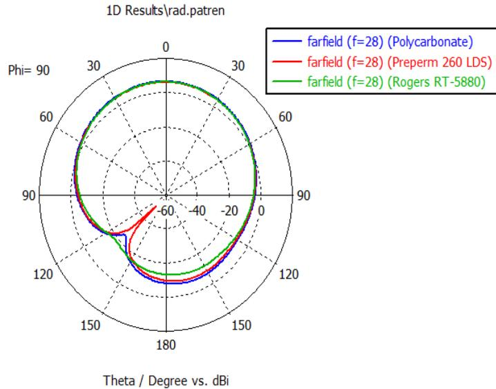
Figure 6. 2-D radiation pattern plot of the three proposed structures.
