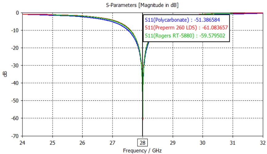
Figure 2.  $S_{11}$  plot of the three proposed structures
