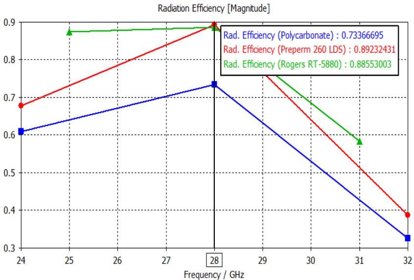
Figure 5.  $\eta_{rad}$  % plot of the three proposed structures
