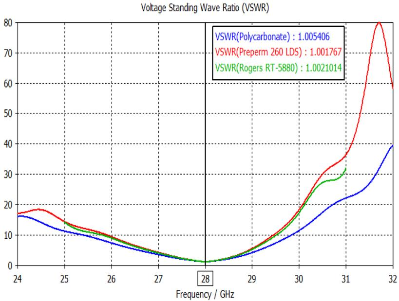
Figure 4. VSWR plot of the three proposed structures
