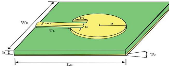
Figure 1. Proposed circular patch antenna structure.
