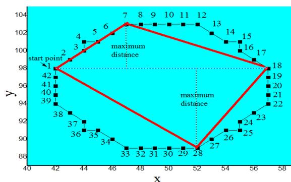
Figure 5. Curve approximation using the Ramer method
