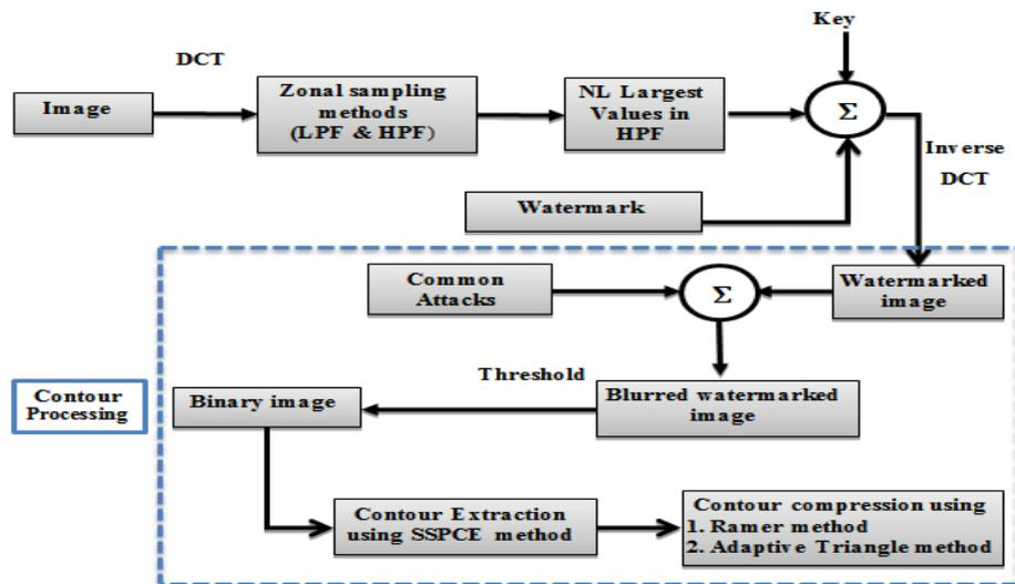
Figure 4. Block diagram of contour extraction using SSPCE and compression using Ramer and Adaptive Triangle methods
