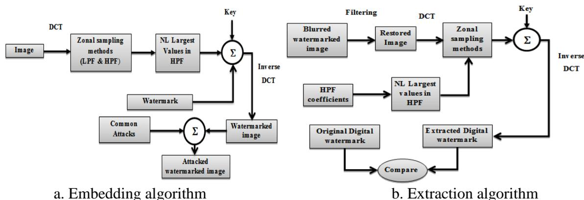
Figure 1. The proposed enhanced watermarking algorithm
