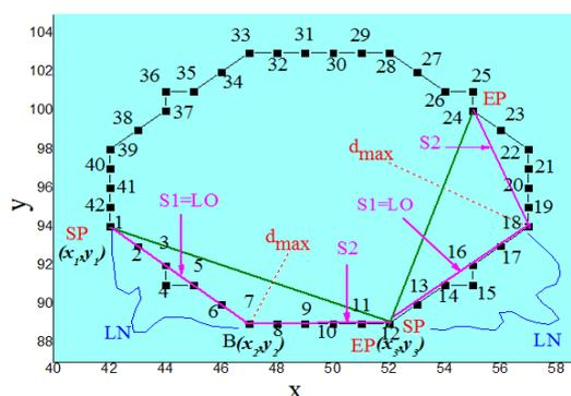
Figure 6. Curve approximation using Adaptive triangle method
