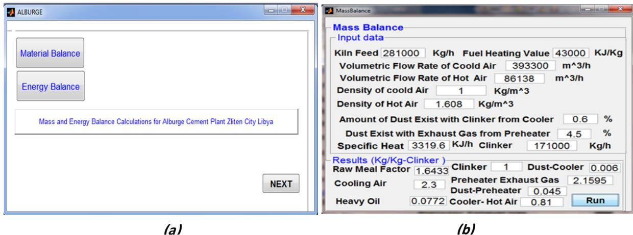
Figure 2. A graphical User Interface (GUI) screens: a) main menu; b) input data for material balance
