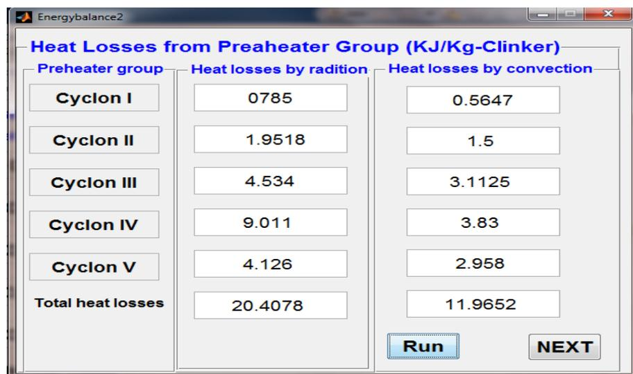
Figure 6. Graphical User Interface Matlab for Calculating heat losses from preheater group
