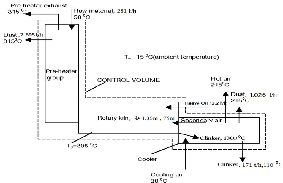
Figure 5: The boundary of kiln system control volume.
