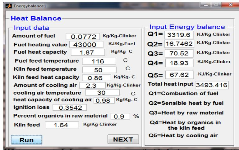
Figure 4. Input data for energy balance
