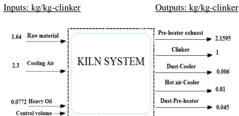
Figure 3. Mass balance of the kiln system.
