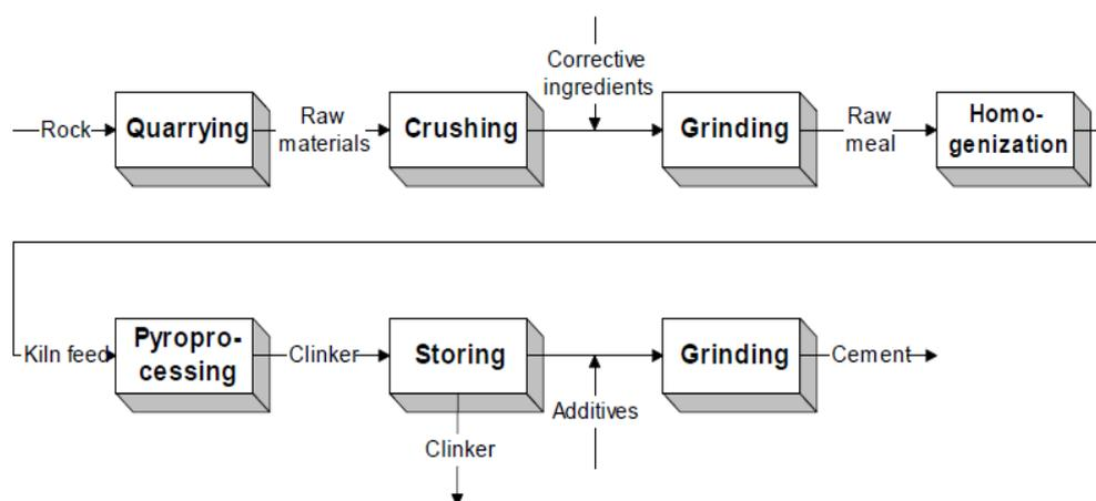
Figure 1. Schematic diagram of cement manufacturing process [9].
