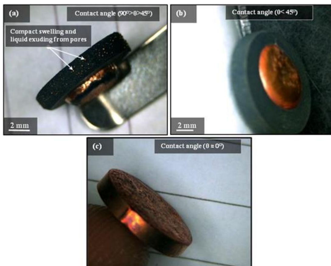
Figure 5. The photographs of 80W-Cu sintered compact at 1150°C under different furnace environment via Cu-MI method: (a) under vacuum, (b) under Ar./H 2 gas (95/5 wt.%) and (c) under H 2 gas
