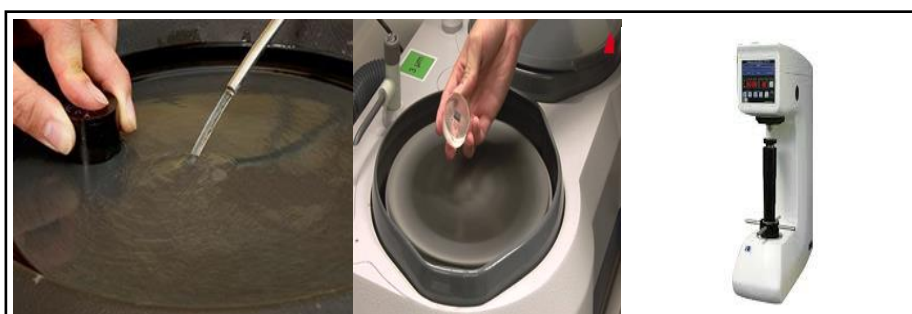
Figure 2 Grinding, Polishing and Micro-hardness measurements
